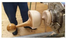
Turn the body, again starting with the roughing gouge, and then using the  $\frac{1}{2}$ " spindle gouge to shape the body and feet, Finish as with the neck, and then part it off.
