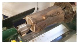
Start with a roughing gouge to take the edges off, then use a <sup>1</sup>/<sub>2</sub>" spindle gouge to start forming the neck. There should be a sharp edge where the body starts, and you need to make a straight right angle cut to achieve this. Mark about <sup>3</sup>/<sub>4</sub>" down to define where the head will be and swap to a 3/8" gouge to
